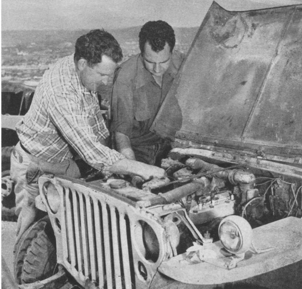
• Vic Hickey and Don Francisco discuss installation of finned aluminum head on Jeep.
